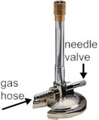
A Bunsen burner is a type of lab equipment used to heat substances by flame. | A Bunsen burner is a type of lab equipment used to heat substances by flame. |
